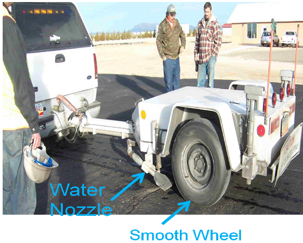
Figure 3.7 Dynatest Skid Resistance Equipment
