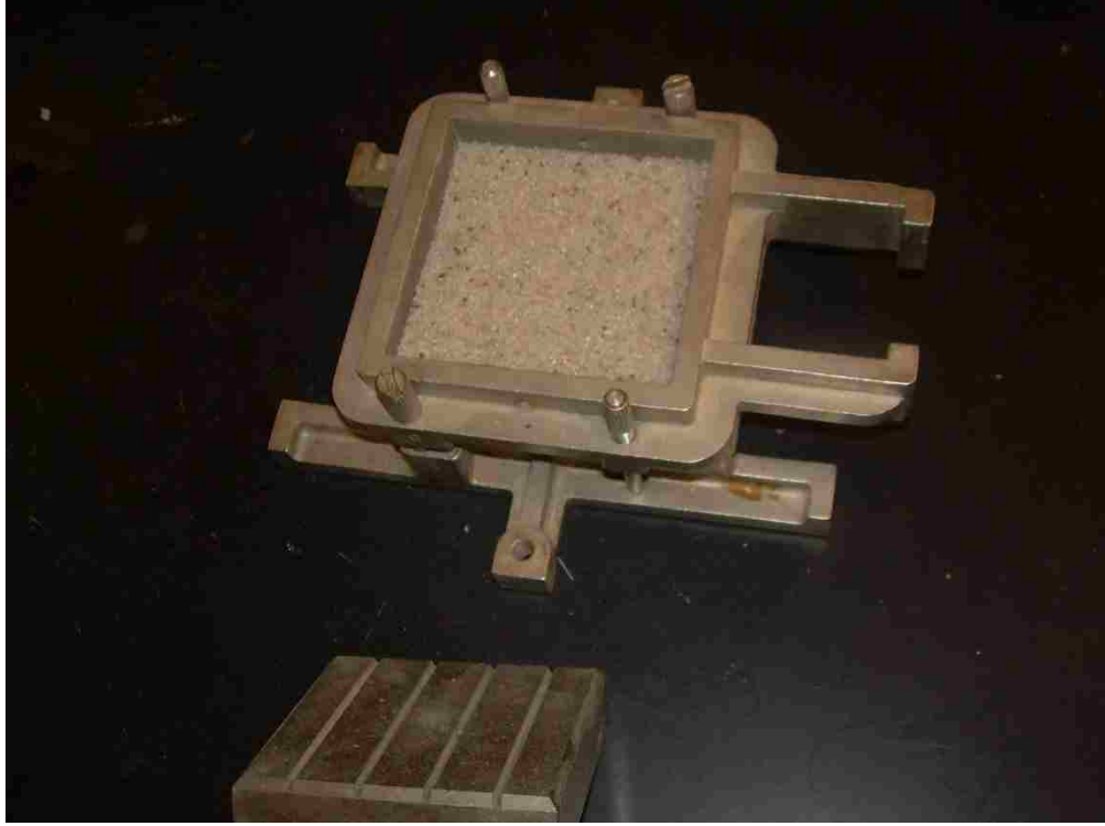
Figure 3.18 Shear Box with Sample
