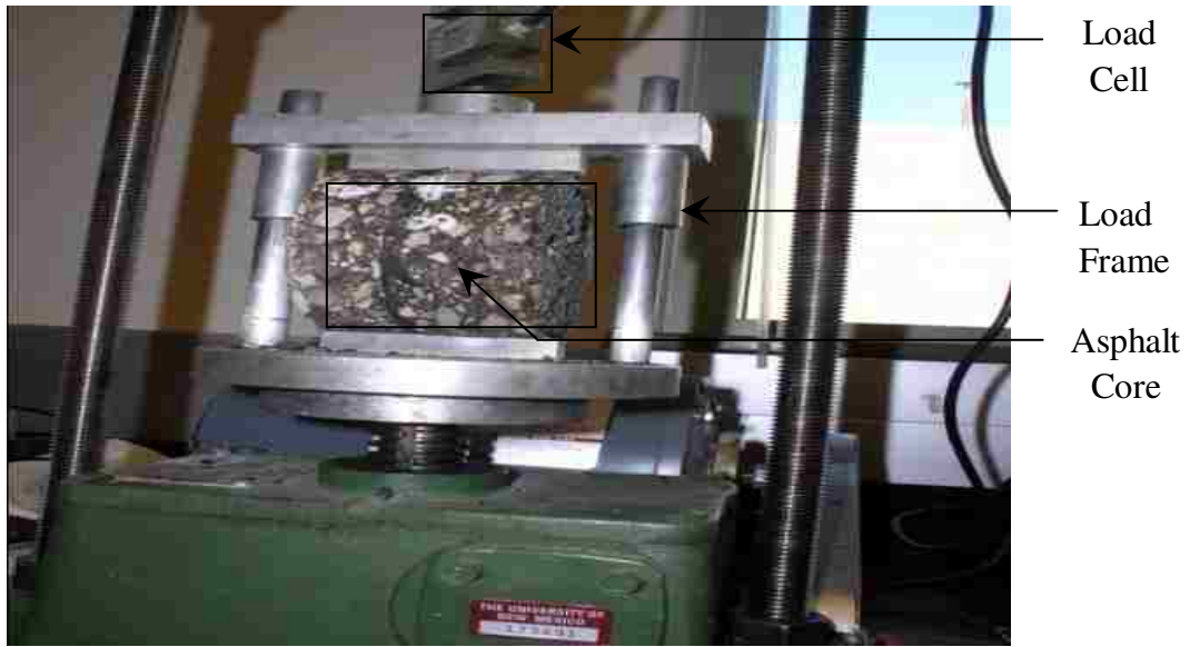
Figure 3.21 Indirect Tensile Strength Test
