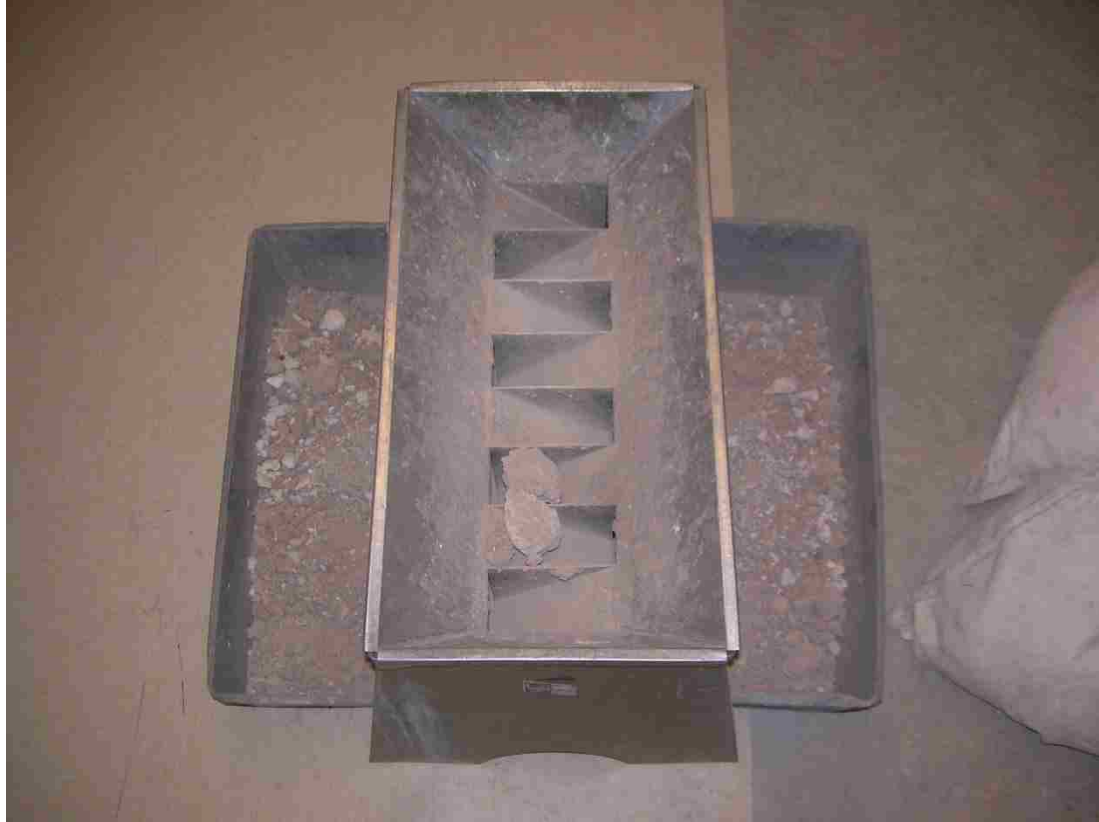
Figure 3.13 Splitting of the Soil Samples
