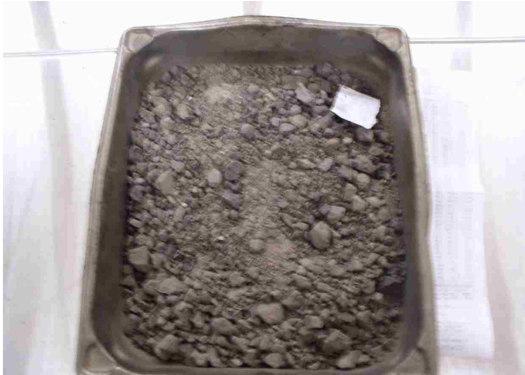
Figure 3.25 Sample for Gradation Analysis after Determination of Asphalt Content
