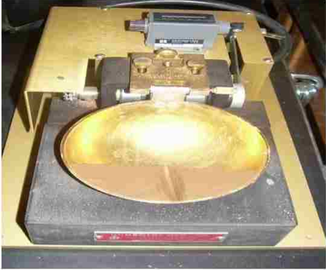
Figure 3.15 Liquid Limit Test
