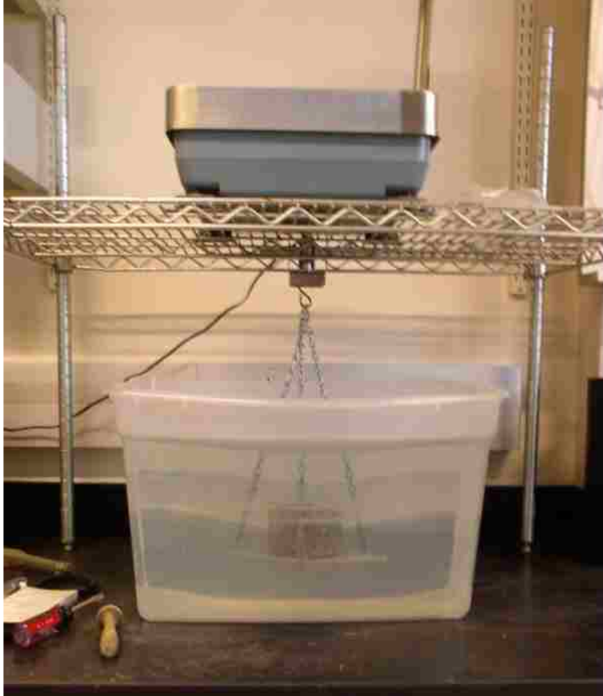
Figure 3.22 Bulk Specific Gravity Test
