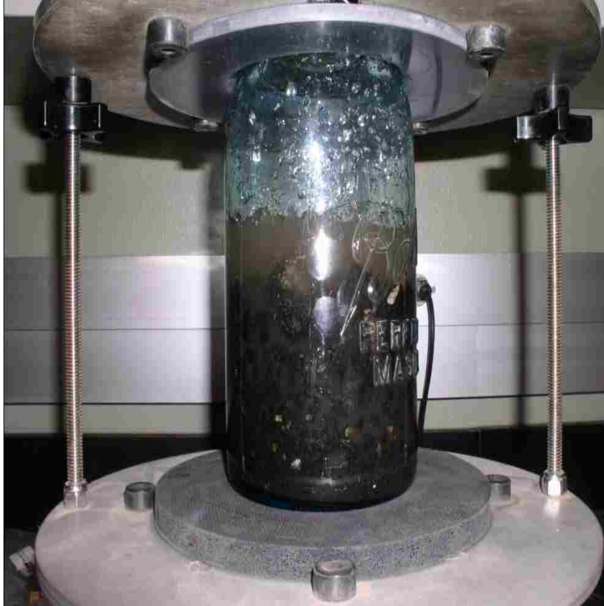
Figure 3.23 Theoretical Maximum Specific Gravity Test
